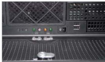
AREMO-4196 is equipped with two USB 2.0 connectors on the front panel to have a better security control.
