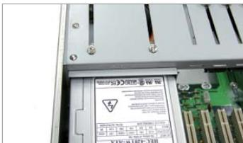
Flexible design to install power supply, the bracket can be adapt to PS/2 type or mini-redundant power supply.
