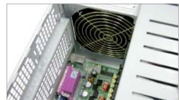
The washable fan filter can be easily taken out for easier maintenance.
