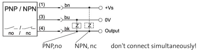
through-beam transmitter, PS12 and PS18
