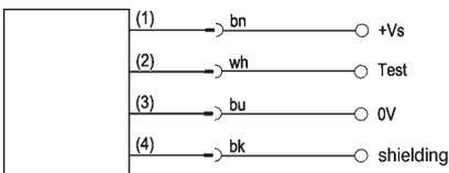
through-beam receiver PE12 and PE18
