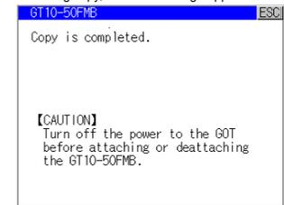
When only the project data was copied to the GOT, touch the [ESC] button to restart the GOT and display the user-created screen. When the standard OS was copied, the GOT will automatically start up and display the user-created screen. (If the project data does not exist, a message appears to notify that the project data does not exist.)
