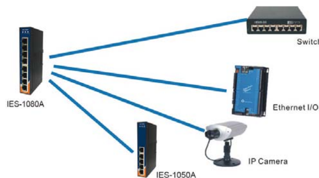
Connections of Ethernet devices
