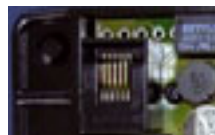
Optional plug-in screw terminal or RJ12 socket
