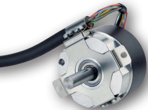
The AD34 is the most compact absolute encoder in class. It is available with a resolution up to 17 Bit Singleturn. The mechanical design consists of two ball bearings and a flexible torque support. The AD34 complements the ACURO-DRIVE series and is appropriate for use within BLDC servo motors with small frame sizes. The AD34 is available with a notched shaft, which saves installation time.
