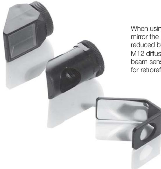
When using the diagonal mirror the sensing range is reduced by 30 % for the M12 diffuse and M12 through-beam sensors. Not suitable for retroreflective sensors.
