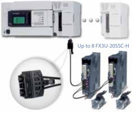
SSCNET communication is simply "plug and play".
